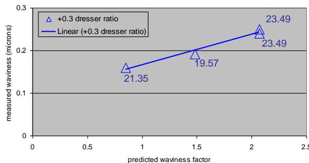
Figure 6. Measured waviness value vs. predicted waviness factor in cylindrical grinding using crude model.
