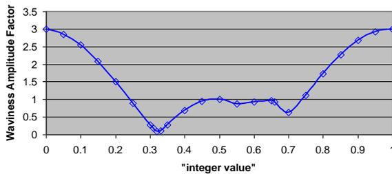
Figure 5. Waviness factor vs. fractional portion of ratio Wheel-RPM/Workpiece-RPM.
