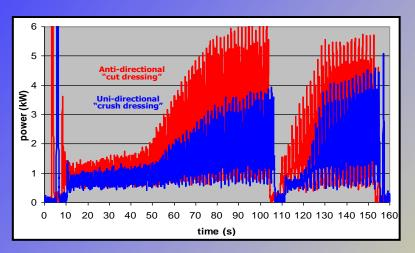
■ Example: Grindometer® output showing the drastic effect of dressing uni-directional vs. anti-directional in continuous-dress creep-feed grinding of nickel-alloy turbine blades.
