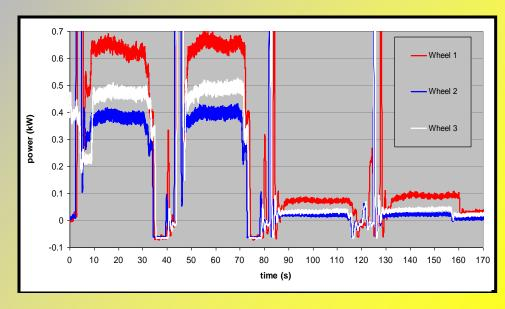
**Example:** Grindometer® output showing the effect of improved coolant nozzles.
