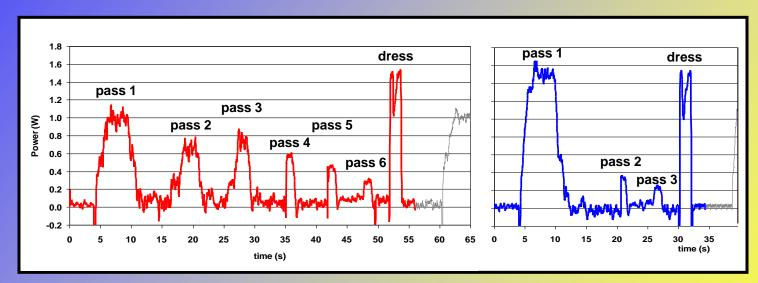
Example: Grindometer® output comparing three different grinding wheels. The wheel generating the lowest power will give the lowest temperatures.
